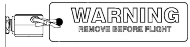
Figure 12. Circuit Breaker Safety Lock Installed with Warning Tag using String/Lacing Tape
