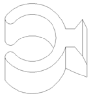
Figure 7. Circuit Breaker Lockout Ring
